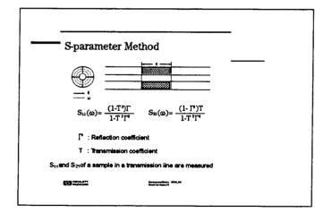
Permittivity and permeability are computed from the measurements of the reflected signal and transmitted signal in the s-parameter method. The reflection coefficient and the transmission coefficient are derived from the s-parameters, length and the input impedance is measured again. Then the Permittivity and permeability are calculated from the two impedance values. S-parameter Method
