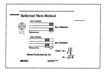
The reflected wave method involves placing the material inside a portion of an enclosed transmission line. The line is usually a section of rectangular waveguide or coaxial airline. In the reflected wave method, the end of the sample is shorted and the input impedance is measured at the reference plane. The sample is moved a quarter of a wave length and the input impedance is measured again. Then the Permittivity and permeability are calculated from the two impedance values.
