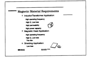
Here are the typical requirements in testing magnetic materials for major applications. Since the operating frequencies of electrical equipment and components is generally going higher, high frequencies are required for magnetic materials. In magnetic head applications, high frequencies are necessary to reach high densities for magnetic recording. By using low loss shielding material, low transmission impedance material can be developed that have high shielding characteristics.
