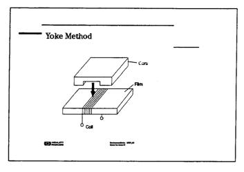
In the voke method, the inductor is wound directly onto a thin film material, and then placed on a core. A high permeability ferrite yoke core is used for this measurement.
