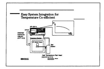
The HP 4291A provides the following features and options to simplify evaluating temperature characteristics.
