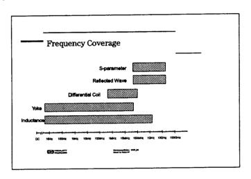
This figure shows the frequency coverage of each measurement method. The inductance and yoke method have wide a frequency coverage, but they can not be used at high frequencies. The reflected wave and s-parameter method is used to test at high frequencies.
