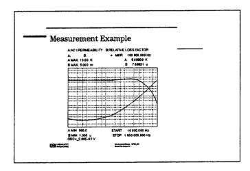
This is a measurement example of initial AC permeability and relative loss coefficient frequency characteristics. Using the auto sequence program (installed in HP4194A, HP4195A) function, it is possible to automatically calculate, display on the CRT and output the test data to a printer the magnetic material frequency characteristics based on an impedance measurement data. Refer to the application note 339 for details.
