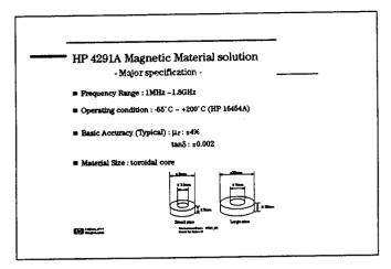
The HP 4291A measures the accurate relative permeability and loss tangent up to 1.8 GHz with the operating condition from -55 degree C to 200 degree C. The HP 16454A comes with two adaptors to accomodate many different sizes of toroidal shaped material.
