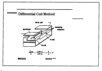
frequencies). where, dVb: Increase in voltage when the material is inserted in the loop
