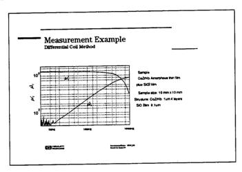
This is an example of a thin film magnetic material measurement by the differential coil method. The sample is a CoZrNb Amorphous thin film with an oxidized silicon base.
