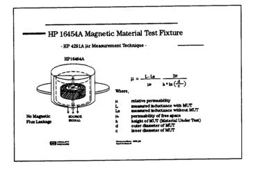
The new HP 16454A test fixture is designed to be ideal structure (no magnetic flux leakage). The relative permeability is derived from the inductance with/without MUT (basically inductor method).
